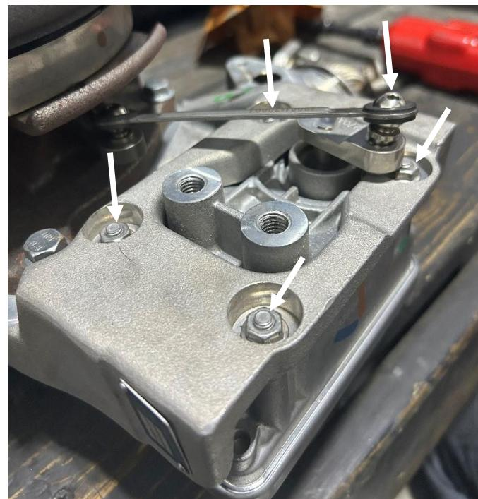
**STEP 45:** Install the OE actuator onto the new Fleece Performance Cheetah turbocharger. Use the four nuts that retained the actuator to the OE turbo to mount the actuator. Torque the four nuts to 93 in-lb.
