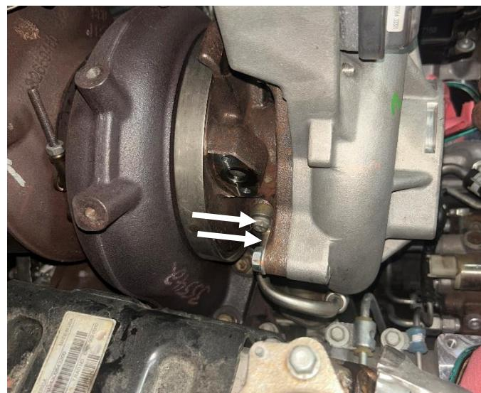
**STEP 35:** Locate the turbocharger oil drain just below the coolant feed fitting removed in step 34. Remove the two bolts retaining the turbocharger oil drain to the engine block using a 10mm socket or wrench.
