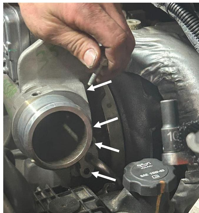
**STEP 38:** Loosen the nut on the turbocharger discharge clamp using an 11mm socket or wrench. Leave the nut three to four rotations from the end of the threaded rod.
