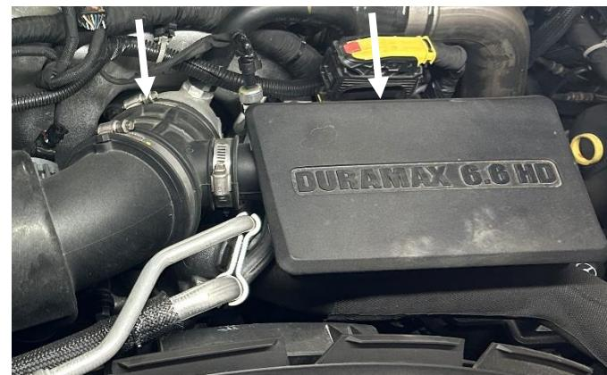
Connect the air filter box and middle intake tube to the boot installed onto the intake horn. Tighten any hose clamps. Install the screws retaining the upper air filter housing.
