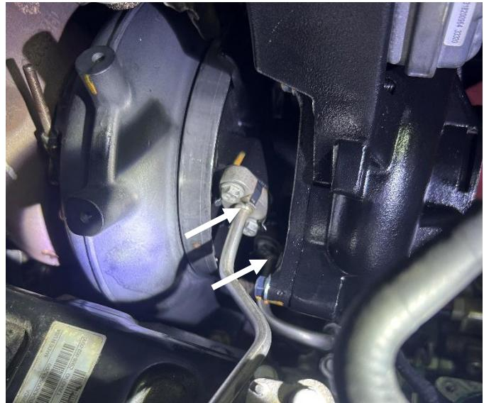
**STEP 55:** Install a new gasket onto the turbocharger oil feed fitting (GM 12737099). The gasket will clip into place on the fitting. Install the fitting into the turbo and use a 10mm socket to torque the two bolts to 89 in-lb.
