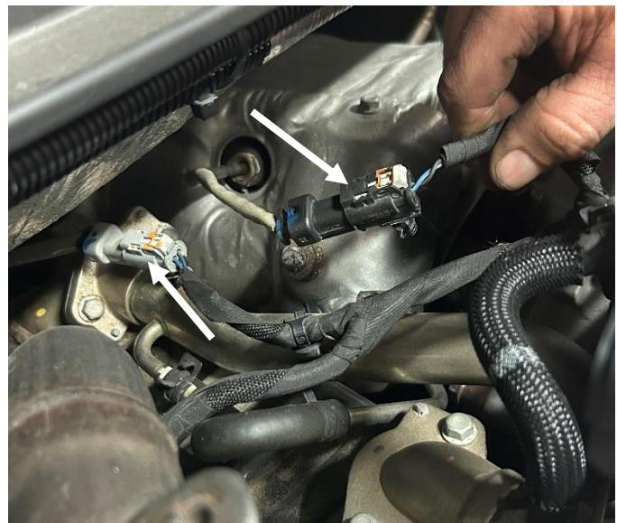
**STEP 20:** Disconnect the harness connector for the EGR mixing valve.
