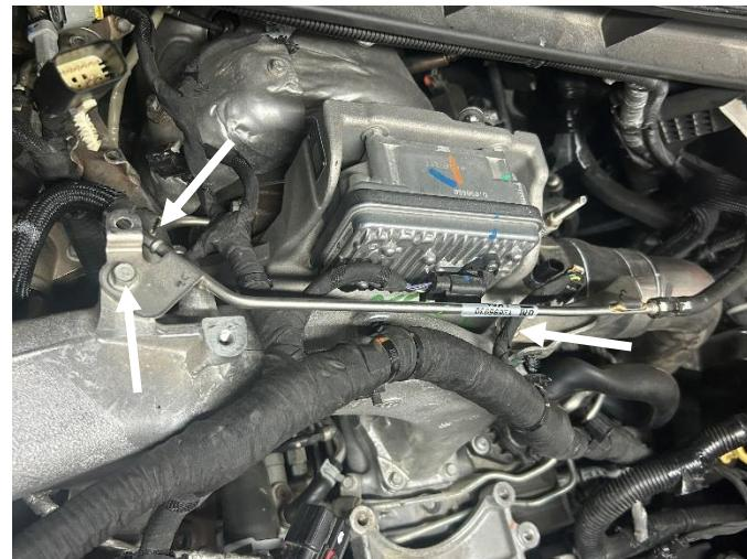
**STEP 22:** Disconnect the harness connectors for the turbocharger actuator and turbocharger inlet air temperature sensor.
