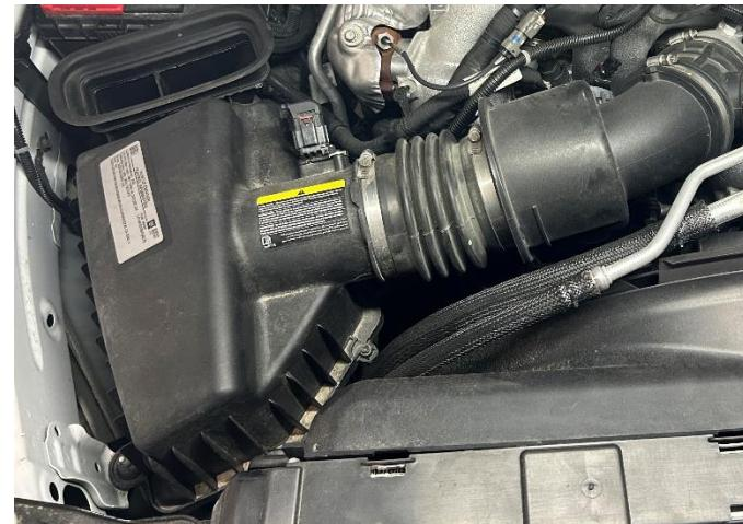
**STEP 90:** Connect the mass airflow sensor.
