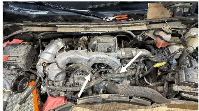
**STEP 26:** With the intake bridge removed, place rags or covers over the intake manifold inlets to prevent foreign debris/objects from entering the engine.
