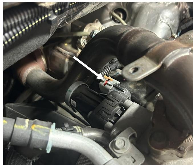
**STEP 21:** Disconnect the coolant hose from the passenger side of the coolant pipe located in front of the turbocharger actuator. Remove the two bolts retaining the coolant pipe to the top of the intake bridge using a 10mm socket or wrench. Place the pipe on top of the coolant tank or set aside.
