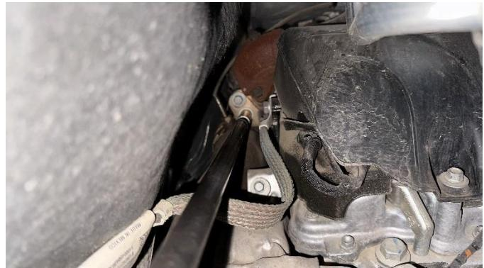
**STEP 6:** Disconnect the harness connectors for the throttle valve and the charge air cooler outlet temperature sensor. Uncouple the charge air cooler outlet tube from the intake bridge.
