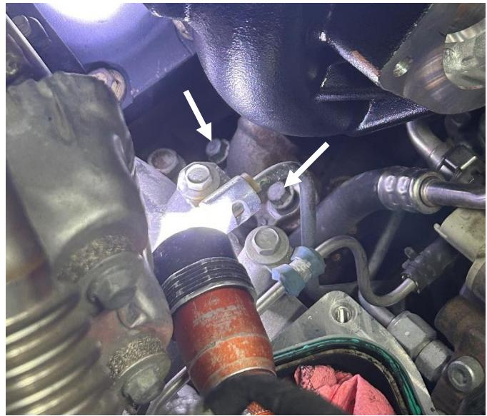
**STEP 54:** Install new gaskets onto the coolant feed and drain connections. Both connectors will use GM 12737099 included in the kit. The gaskets will clip into place on the fittings. Install the coolant feed (lower) first, then the return (upper). Using a 10mm socket, torque the bolts (two per fitting) to 89 in-lb.
