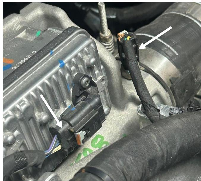
**STEP 23:** Disconnect the harness connector for the coolant temperature sensor located near the passenger side of the A/C mounting bracket.
