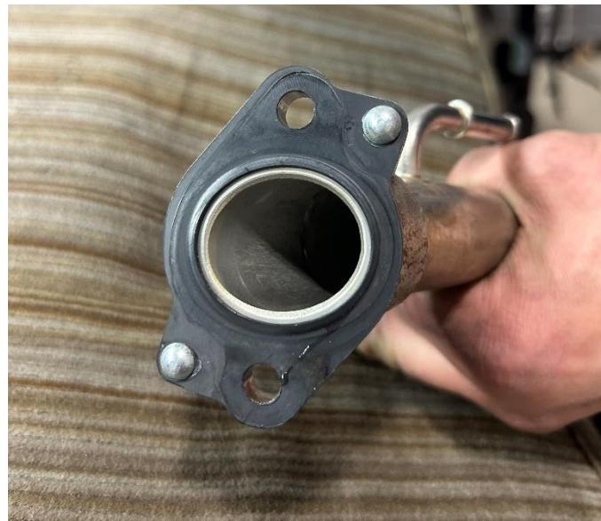
**STEP 64:** Install the EGR coolant pipe as shown at right. Using a 10mm socket or wrench, torque the two bolts to 89 in-lb. Connect the turbocharger coolant return hose to the barb on the pipe. Fasten the hose clamp.
