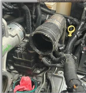
**STEP 32:** Remove the SCR heat shield.
