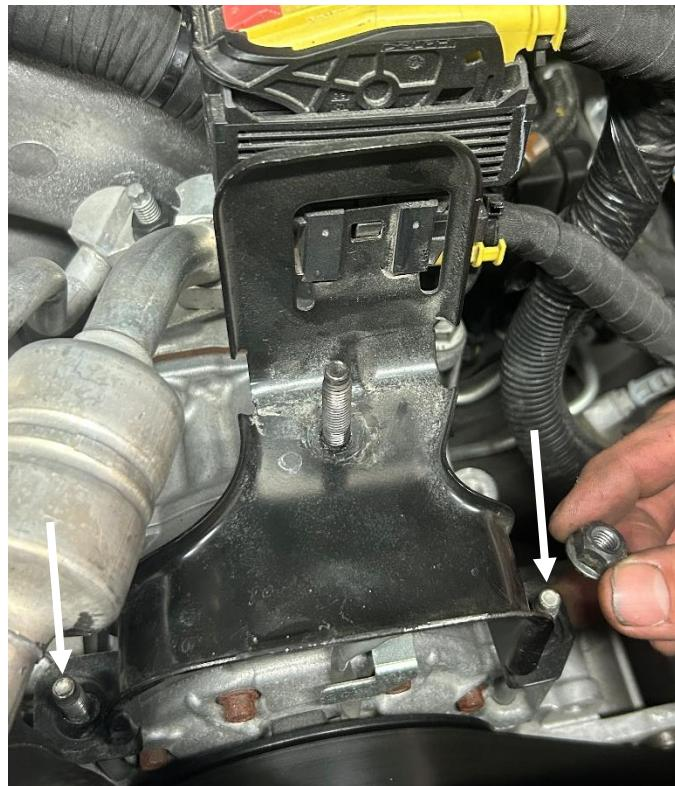
**STEP 14:** Disconnect the two harness connectors located on the driver's side of the A/C compressor.
