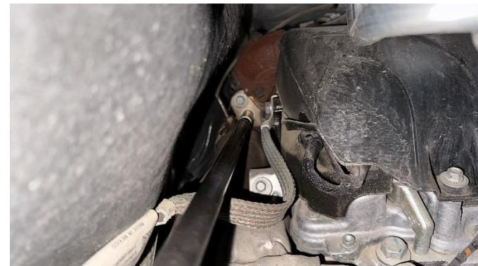
**STEP 92:** Connect the lower radiator hose to the radiator and fasten the hose clamp.
