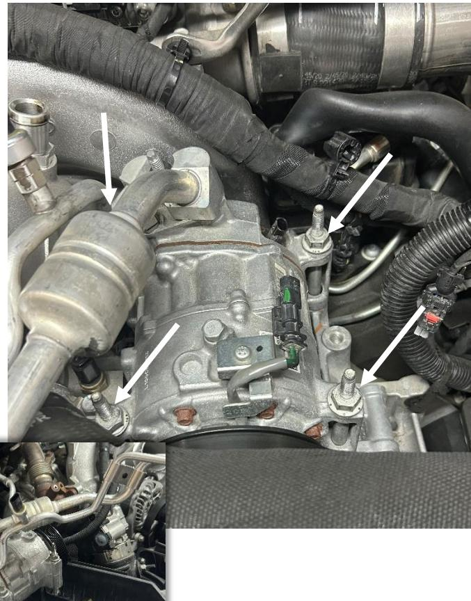
**STEP 16:** Remove the four bolts retaining the A/C compressor to its mounting bracket using a 15mm socket or wrench. Set the A/C compressor aside without disconnecting the hoses as shown at right.
