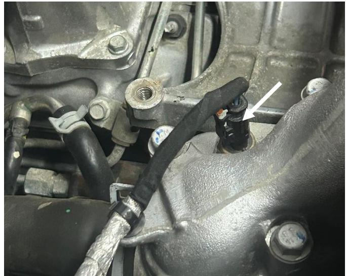
**STEP 24:** Carefully remove any zip ties and fir trees retaining the electrical harness to the intake bridge. Position the harness towards the front of the engine bay to make room for the remaining disassembly steps.
