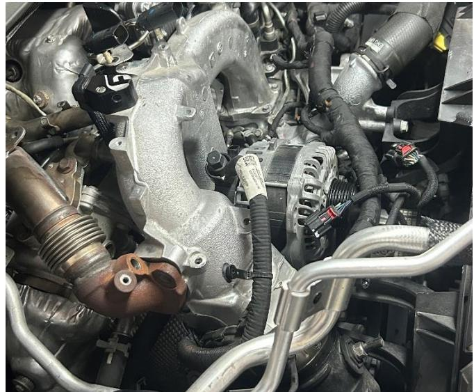
**STEP 69:** Carefully place the intake bridge onto the intake manifolds. Using a 10mm socket or wrench, torque the eight bolts to 89 in-lb.
