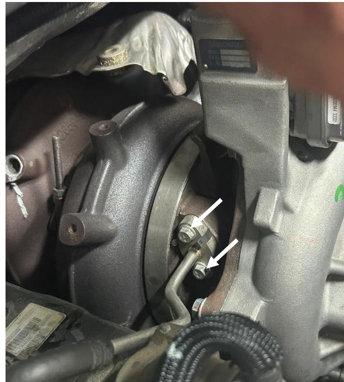
**STEP 34:** Remove the two bolts retaining the turbocharger coolant feed fitting using a 10mm socket or wrench. Move the fitting away from the turbocharger. Remove and discard of the gasket.
