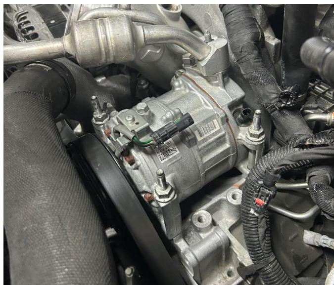
**STEP 77:** Connect the two harness connectors on the A/C compressor.
