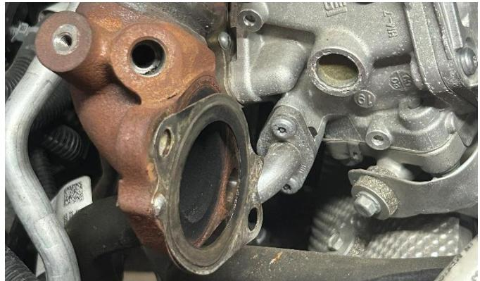
**STEP 68:** Remove any rags or covers placed in the intake manifolds. Ensure that the intakes are free of debris or foreign material.
