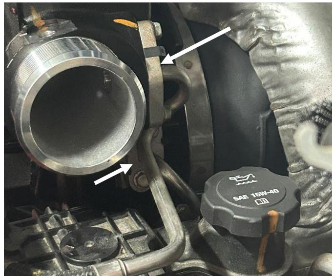
**STEP 57:** Position the driver's side of the SCR heat shield back into place and install the two bolts using a 10mm socket or wrench. Torque the bolts to 89 in-lb.
