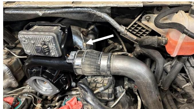
**STEP 63:** Remove the old gasket from the EGR coolant pipe and hose removed in step 28. Refer to the procedure outlined in step 47 to remove and install the new gasket. Use the included gasket P/N GM 12648141.
