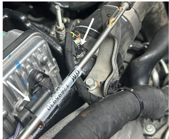
**STEP 73:** Connect the SCR temperature sensor, post-SCR temperature sensor, and the EGR mixing valve connectors.
