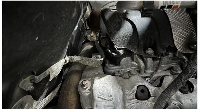
**STEP 5:** Remove the 13mm bolt located behind the center of the resonator. Loosen the hose clamp connecting the intake tube to the intake horn. Disconnect the mass airflow (MAF) sensor. Remove the bolts retaining the upper half of the airbox. Remove the intake and upper airbox.
