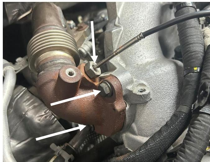
**STEP 83:** Install the EGR temperature sensor. Using a 17mm wrench or flare nut socket, torque the sensor to 33 ft-lb.
