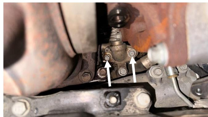
**STEP 36:** Remove the two bolts retaining the PCV tube and fitting to the rear of the turbocharger outlet using a 10mm socket or wrench. Remove and discard of the gasket.
