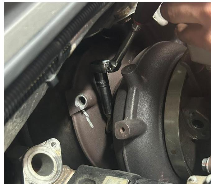
**STEP 39:** Remove the four bolts retaining the turbine housing to the exhaust up pipe using a 15mm socket or wrench. The four bolts are stainless steel and are not magnetic. A grabbing tool may be required to lift the bolts out of the mounting holes once fully loosened.
