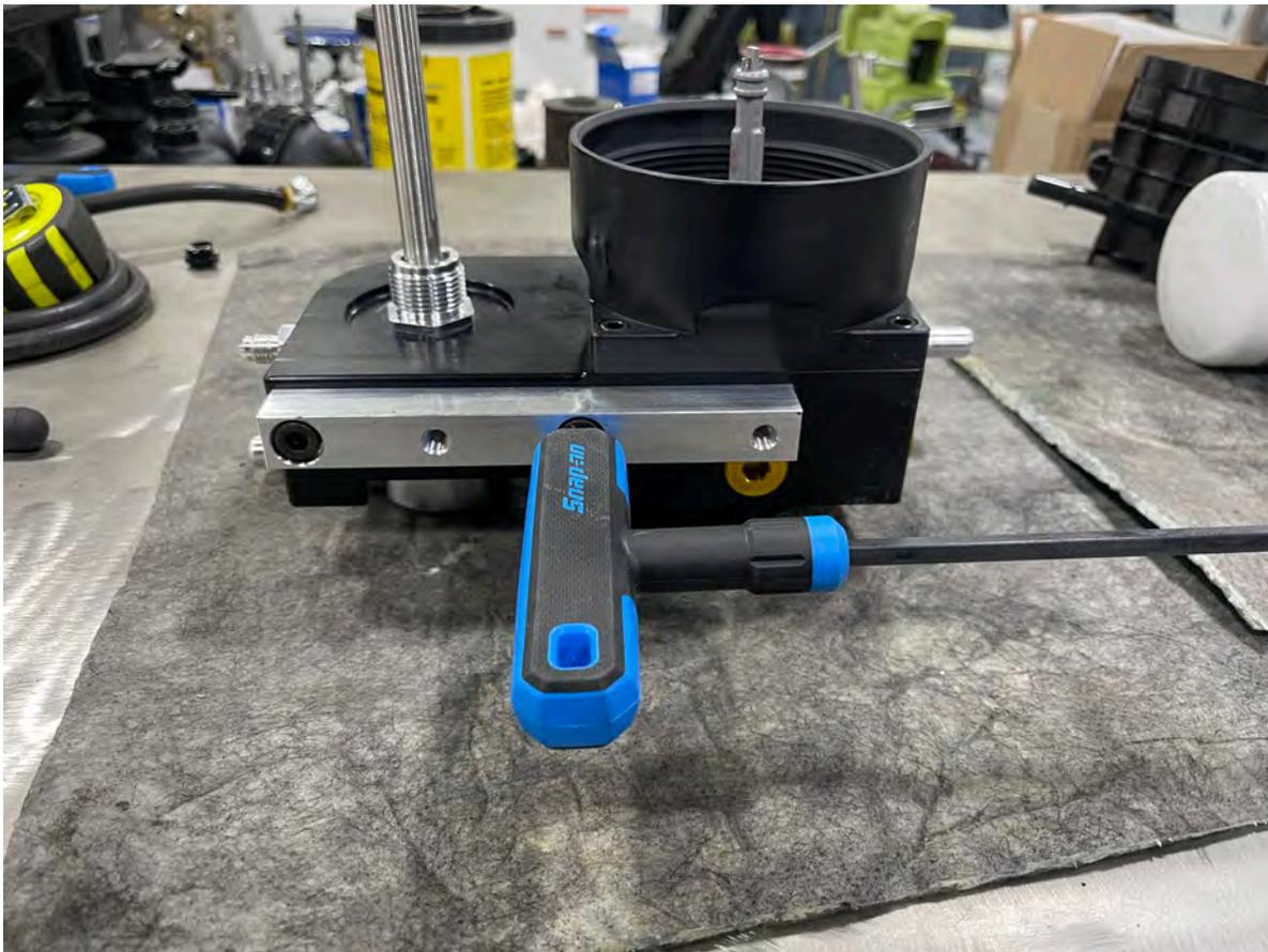
**J. Apply thread tape to the threads of PL-1011, place into 375-QC-1E-NPT and tighten accordingly.**
