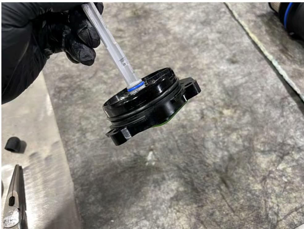
**G. Before installing the WIF sensor, thoroughly grease the o-ring. Using the three supplied allen screws, slowly secure the WIF sensor in a circular pattern until the WIF sensor is fully seated. **NOTE THE LOCATION OF THE WIF SENSOR CONNECTOR!!****
