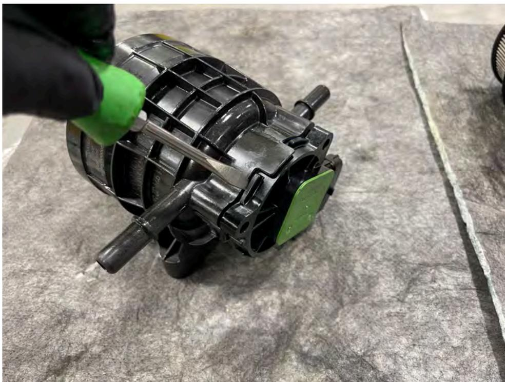
**F. Remove the old WIF sensor o-ring and replace it with the supplied o-ring.**
