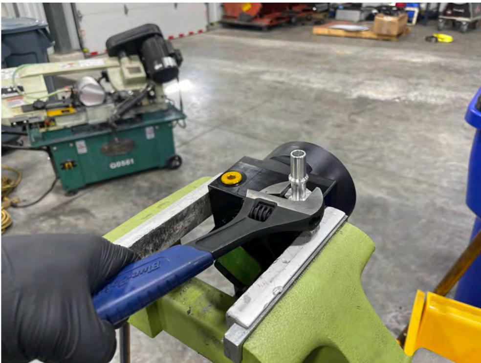
I. Using the two supplied 8mm bolts, secure L5P-ADP-BRK-1001 to the filter base as shown. Tighten accordingly.
