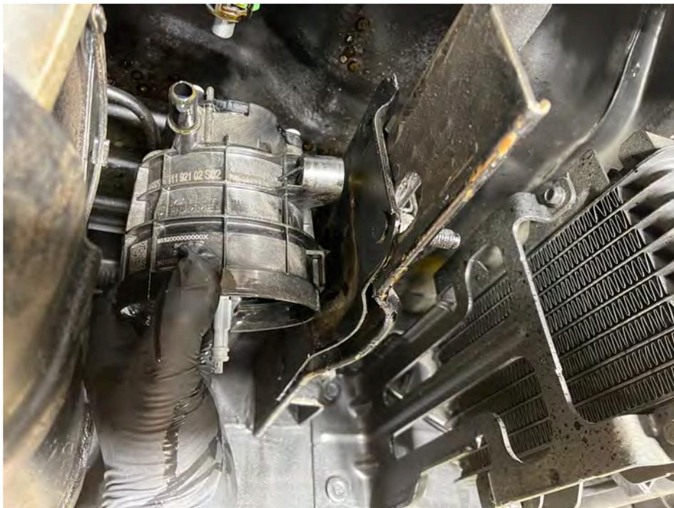
**E. Remove the three torx screws from the WIF sensor, then gently remove the WIF sensor from the filter housing.**
