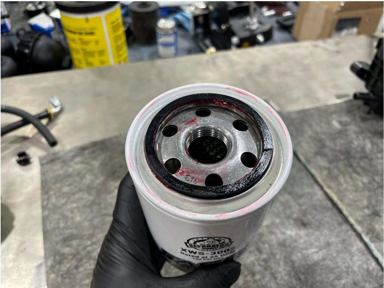
**Q. Install a new water separator into the FASS System, be sure to grease the o-ring prior to installation. Tighten accordingly.**
