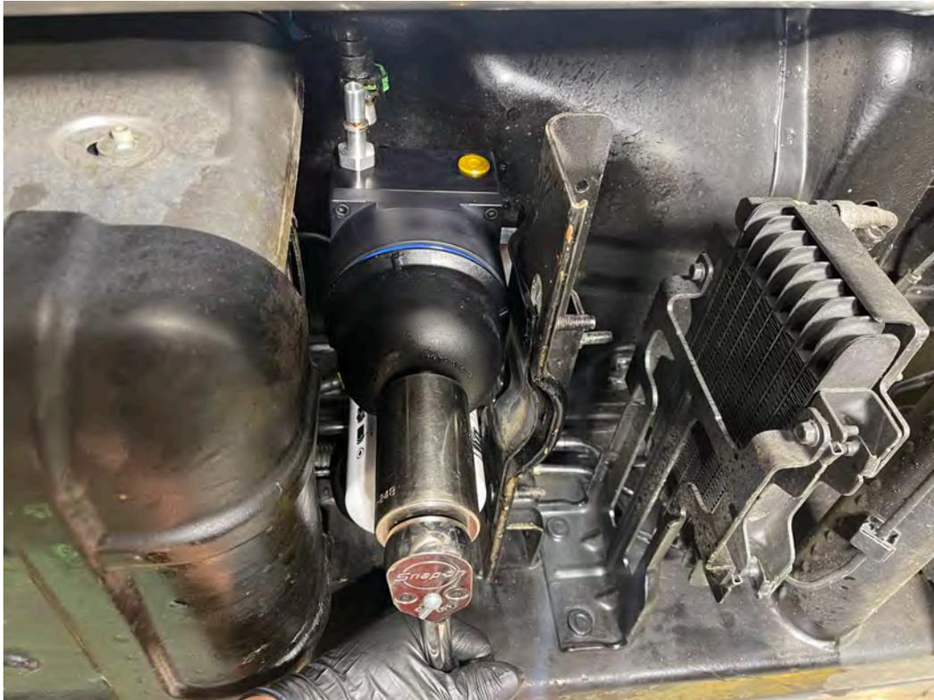
**R. Connect the fuel inlet line to the 8-ORB-500-QC and secure the locking clip.**
