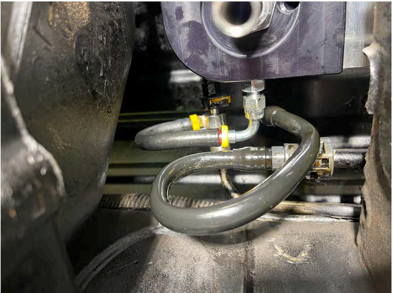
**O. Connect the engine feed line to 10-ORB-500-QC. It might be necessary to disconnect the small plastic section of line from the frame-mounted hard line to get it to connect to 10-ORB-500-QC. Be sure both locking clips are secured.**
