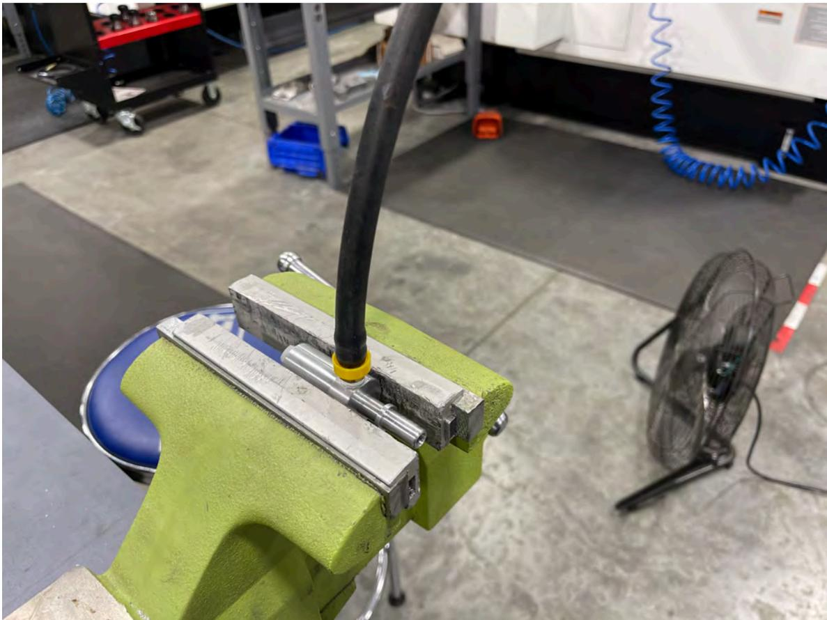
**L. Install 375-QC-1E-NPT onto the fuel return line as shown. Be sure the locking clip is fully seated on the fuel line after it is installed!**
