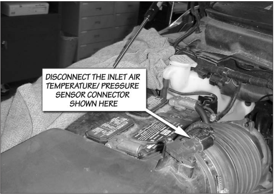
Figure 1 Location of the Inlet Air Temp/Pressure Sensor
