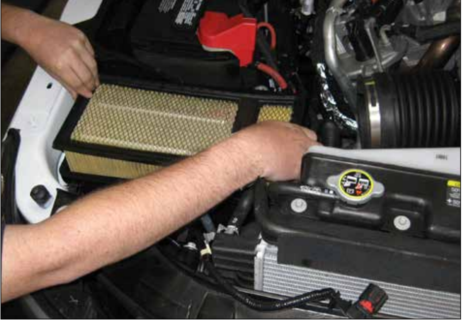
Figure 5-Removing stock air filter element
