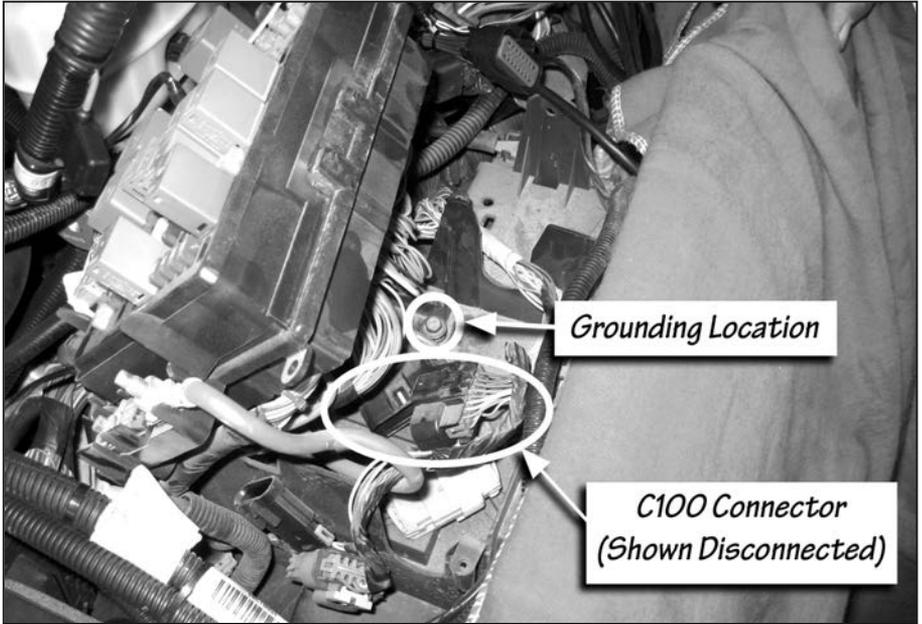
**5.** Secure the wire harness using some of the supplied cable ties along the factory wire harness up the left side of the engine to the Fuse box.
