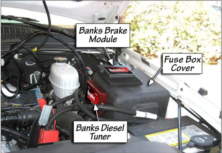
**WARNING: Make sure to place the Banks Brake Module as shown in Figure 11 to avoid a clearance issue when closing the hood. Mount the SpeedBrake Module as close to the inside edge of the fuse cover as possible.**
