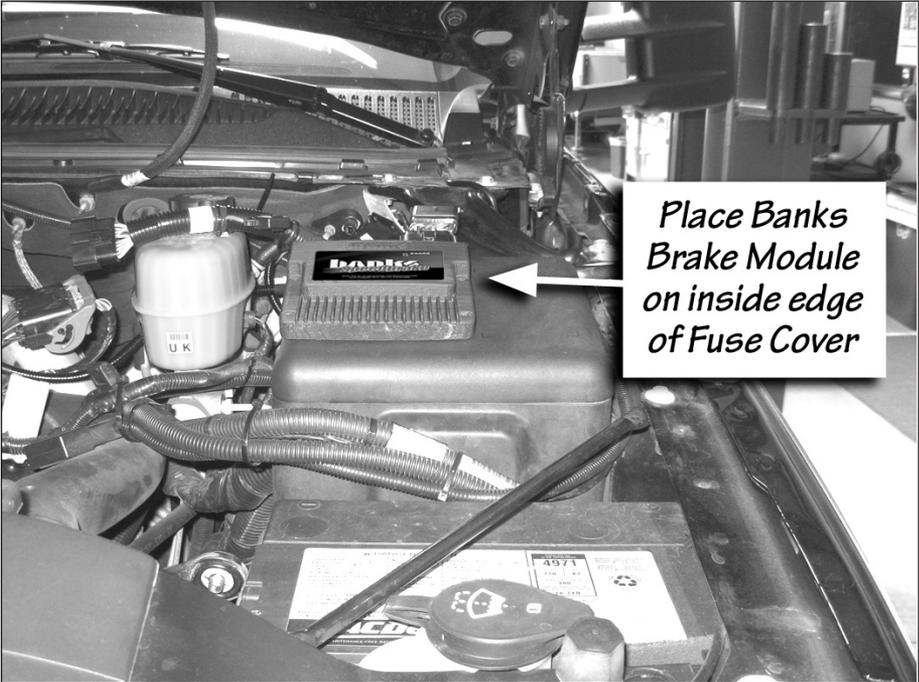
**Figure 12** Placement of Banks Tuner on top of the Fuse Box.
