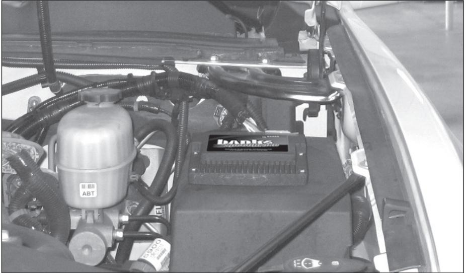
*If vehicle is equipped with a Banks Tuner, the Banks Brake can be installed next to the Banks Tuner.*
