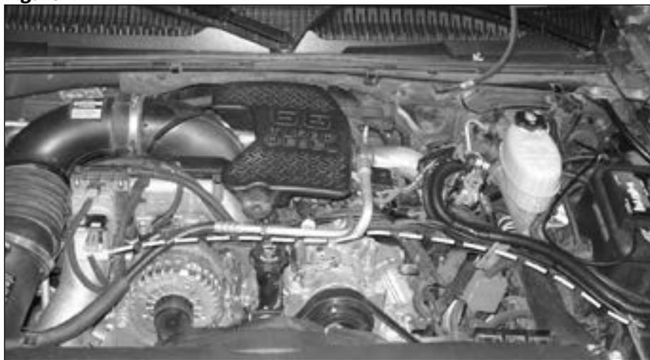
**6.** Locate the MAF connector from the Six-Gun Tuner harness and route as shown in **Figure 4**. Follow the factory harness located on top of the engine that runs in front of the intake manifold and behind the alternator. Feed the connector under the compressor outlet and under where the air intake hose normally rest. See **Figure 5**.
