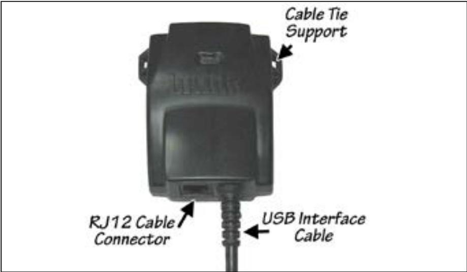
**11.** Route the Banks iQ USB interface cable from the Banks iQ Bridge Module under the dash and out through the fuse access panel opening. The cable can be slid under the door frame's seal and run up to the top of the dash. Pull enough cable to reach the Banks iQ and connect it to the USB receptacle on the left side of Banks iQ. See **Figure 8**. Snap the fuse access panel back in place making sure not to pinch the wire.
