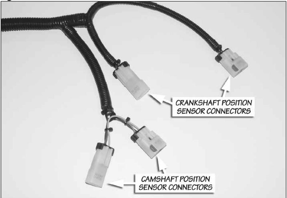
**13.** Locate the Camshaft Position (CMP) sensor below the fuel injection pump between the timing gear cover and the ECM. Unplug the factory connector and plug it into the corresponding male CMP sensor connector on the Six-Gun/EconoMind harness. Plug the Six-Gun/EconoMind's female CMP sensor connector into the sensor. See **Figure 9**.
