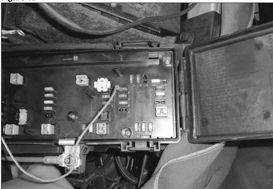
stressed wire. Locate the RED/WHT wire with the Power Terminal on the Six-Gun/EconoMind tuner wire harness and connect it to the mini-fuse blade tap. Replace the fuse cover and make sure not to pinch the RED/WHT power wire.
