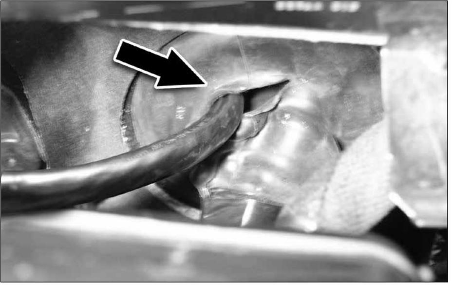
**5.** Remove the electrical connector bracket on the left hand side of the support below the steering column in front of the firewall by removing the two (2) bolts. This will allow access to the inner grommet. See **Figure 4**.
