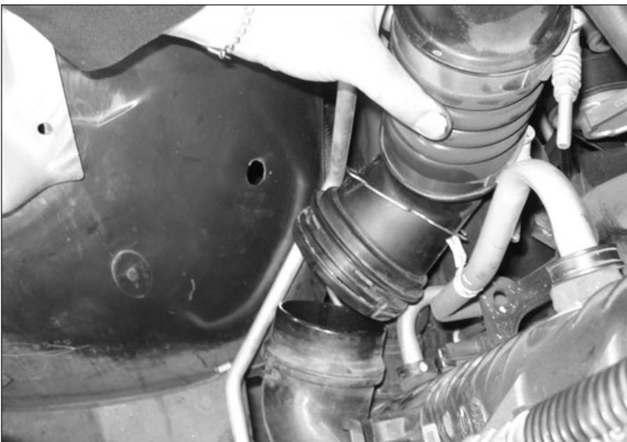
**23.** Loosen the driver side boost tube hose clamps. Remove the boost tube off the charge air cooler (CAC). Do not damage the hoses that attach to the charge air cooler (CAC) as it will be reused. Cover the hose opening to prevent foreign debris from entering. See **Figure 2.14**.
