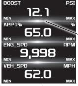
The separator lines will change from Red to **Green**, which indicates that the device is actively recording (datalogging).
