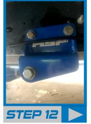
With all 4 holes drilled re-torque the ½" bolts to 30 ft-lbs.
