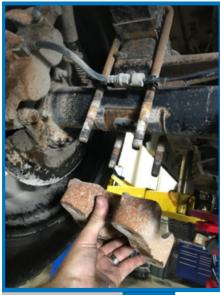
Remove the nuts from the U-bolts. It is recommended to do one side at a time to avoid the axle from shifting. With the nuts removed slide the lower plate off the U-bolts.
